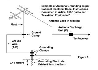
A) Use No. 10 AWG (5.3mm2) copper, No 8 AWG (8.4mm2) aluminum, No. 17 AWG (1.0mm2) copper clad steel or bronze wire, or larger, as ground wire.
